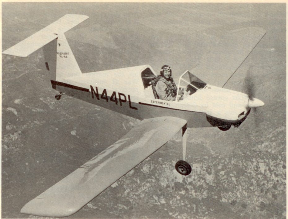
Pazmany PL-4A, with Pete Girard at the controls. A canopy was subsequently added to this homebuilt. The design has created much interest within the homebuilders' ranks. The aircraft is powered by a Volkswagen engine. Photo courtesy of designer
